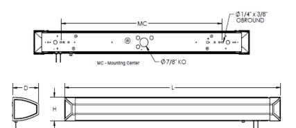
while the longer fixtures provide 1800 source lumens upward and 3600 down. Four position pull switch(on up, on down, on both, all off) are standard and located near the right side of the fixture. LED nightlight with on/off control pull-switch is included.
