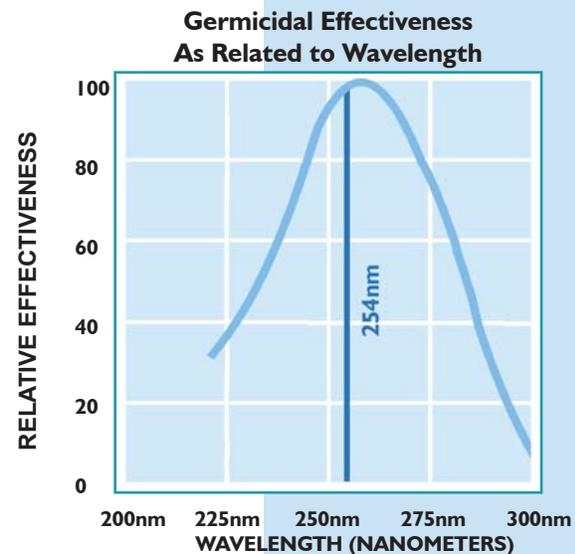
Approximately 95% of the ultraviolet energy emitted from **STER-L-RAY™** germicidal lamps is at the mercury resonance line of 254 nanometers, the region of germicidal effectiveness most destructive to bacteria, mold and virus.
