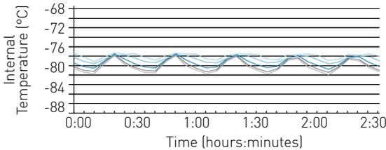
As interior air temperature stabilizes at the desired setpoint, mass storage volume sustains tight temperature uniformity of the load inside the insulated cabinet.
