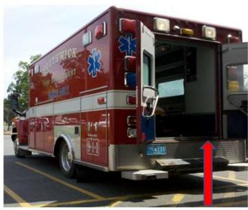
Maximum Loading Height Measured From Ground to Loading Platform
